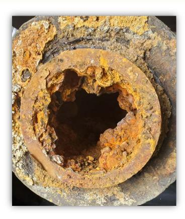
Sediment Buildup & Corrosion of Aging Waterlines
